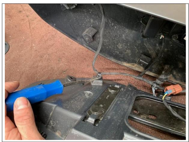
11. Remove all retaining clips for wiring.
