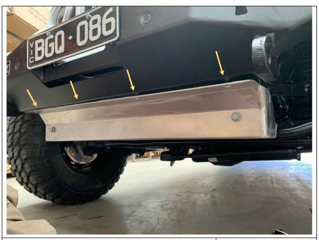
30. If fitting optional skid plate, hold plate up to bottom of bull bar and start the 4x M8 x 30 button head bolts with washers to hold plate in place, and re use hardware for the rear.
