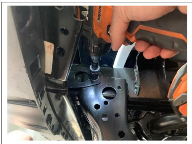
5. Remove reinforcement bracket as shown on both sides.
