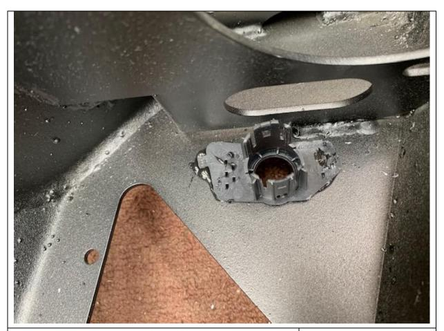
14. Stick housings to inside of bull bar paying special attention to sensor wire orientation. Dry fit and make sure all sensor wires can reach before gluing.
