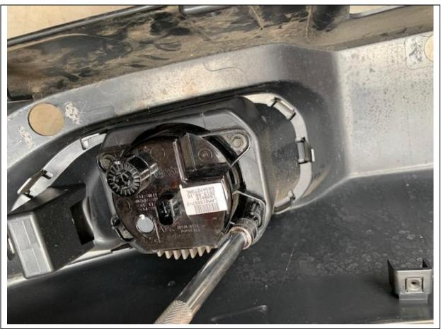
16. Remove factory fog lights from bumper with 8mm socket.
