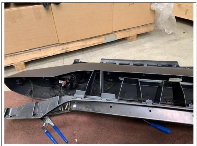
10. Once all screws have been removed, you'll need to separate the inner bumper from the outer shell.
