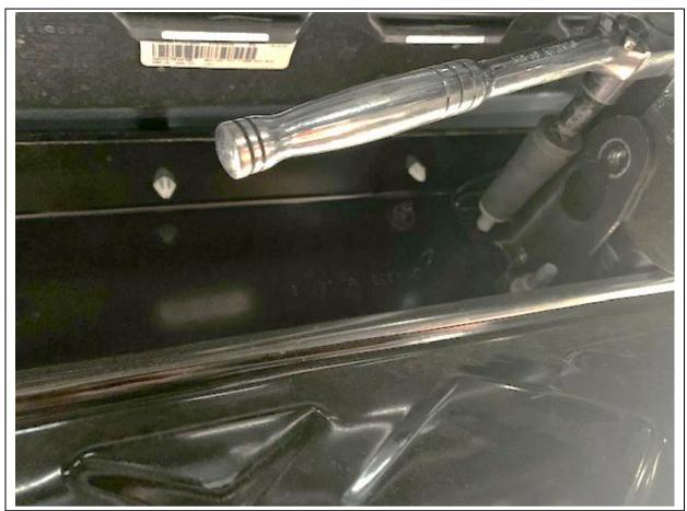
6. Remove 8x 16mm hex nuts securing front crash beam to chassis.
