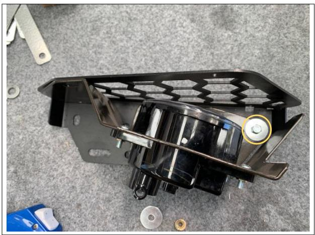
19. Fit fog light bracket to mesh panel like shown using 1x M8x25 hex bolt, flat washer and flange nut. Repeat for other side.
