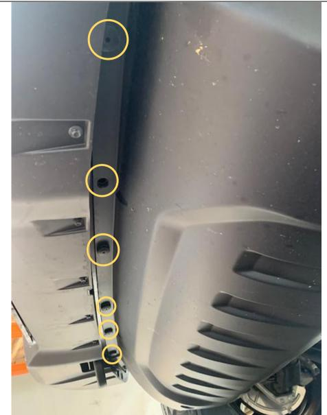
2. Remove all clips from under bumper holding plastic splash guard.
