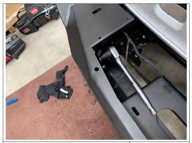
23. Insert 4x M10x30 hex bolts with M10 spring washers and flat washers through chassis into bull bar and torque to 60Nm. Repeat for other side.
