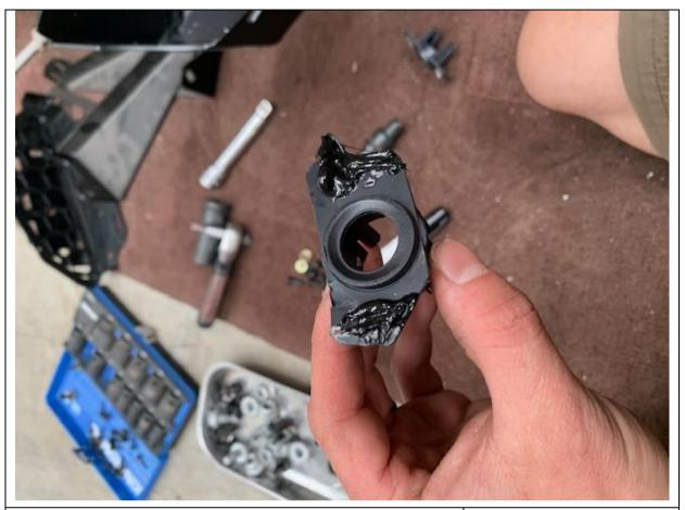
13. To refit the sensor to the bull bar, you'll need to dab the front of the housing like shown with adhesive silicone.
