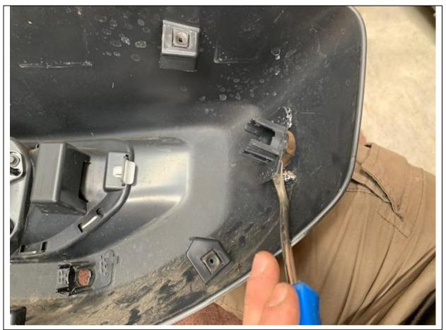
12. If parking sensors are fitted, you'll need to pry the housings off the bumper shell. Make sure you remove the sensors first.
