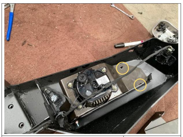
20. Fit mesh panel and fog light to bar and secure each one with 4x M6x16 black button head bolts, black washers and flange nuts.
