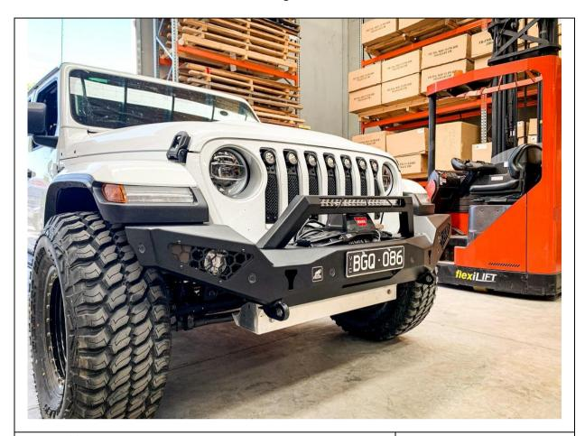
32. If fitting optional stealth hoop, do so now with Supplied M10 hex bolts and Nyloc nuts. You can also fit any 20-22" LED single row light bar at the same time.
